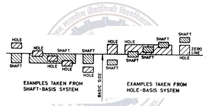
A fit is indicated by the basic size common to both components, followed by symbol corresponding to each component, the hole being quoted first.
