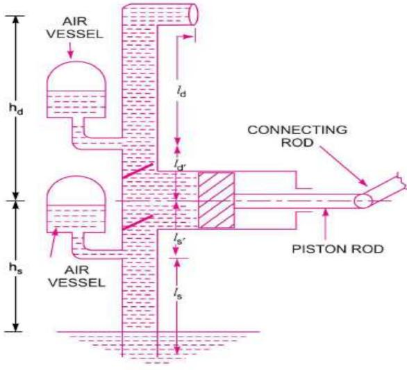
Fig. Air vessels fitted to reciprocating pump.
