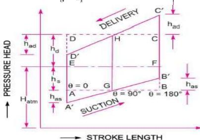
Fig. Effect of acceleration on indicator diagram.
