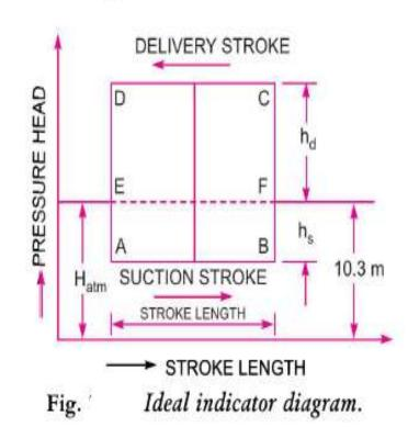
During suction stroke, the pressure head in the cylinder is constant and equal to suction head  $(h_s)$ , which is below the atmospheric pressure head  $(H_{atm})$  by a height of  $h_s$ . The pressure head during suction stroke is represented by a horizontal line AB which is below the line EF by a height of  $h_s$ .
