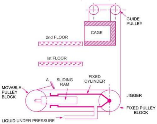
Fig. Suspended hydraulic lift.
