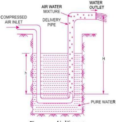
Fig. Air lift pump.
