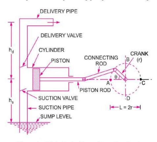
Fig. 1 Main parts of a reciprocating pump.
