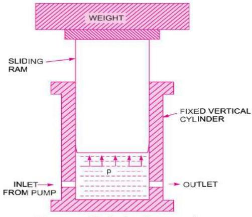
Fig. The hydraulic accumulator.
