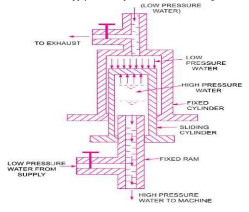
Fig. The hydraulic intensifier.
