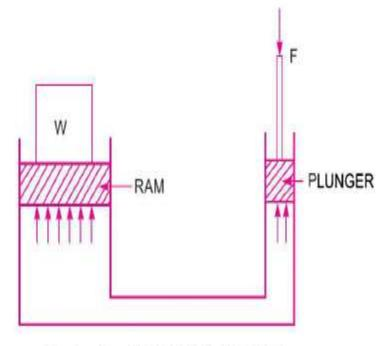
Fig. 1 The hydraulic press.
