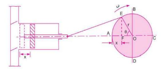
Fig. Velocity and acceleration of piston.
