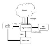
Figure: 6 Web Crawling Working process
