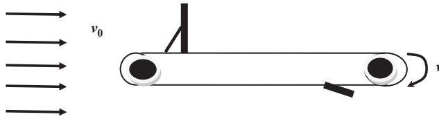
Figure 7.18 View of drag machine with hinged flaps on rotating belt.
