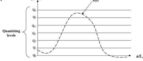
Figure.(2) A sampled signal and the quantized levels
