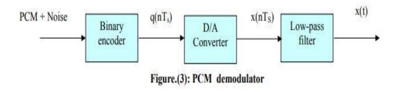
• The choice of the parameter for the number of quantization levels must be acceptable with the quantization noise (quantization error).
